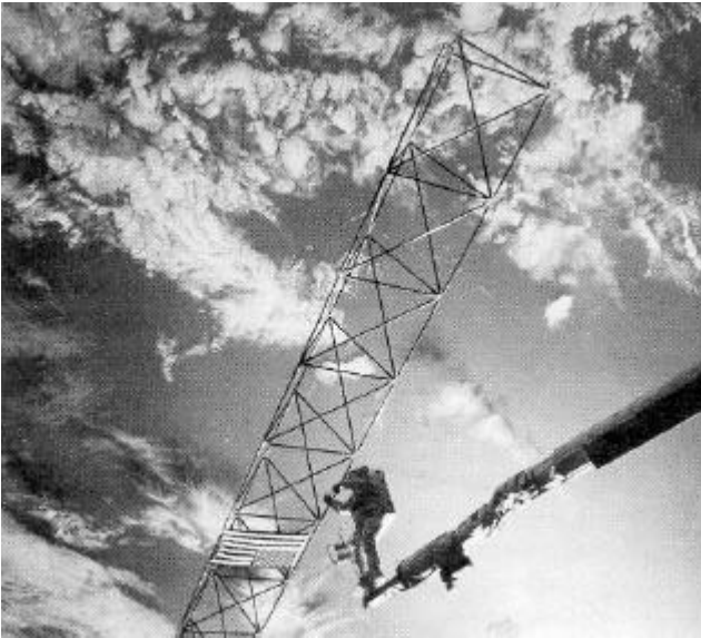
Astronaut Sherwood C. Spring wears the EMU while checking joints on a tower extending from the Space Shuttle Atlantis cargo bay during mission STS 61 -B. He is standing on the end of the arm of the remote manipulator system connected to the space shuttle.
